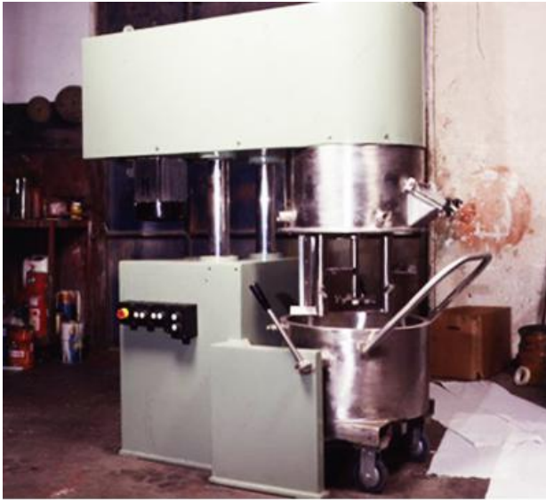
PDP Planetary Mixer with Movable Can
